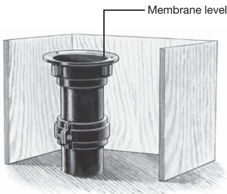
4. Connect body (with spigot adaptor if applicable) to pipework.
