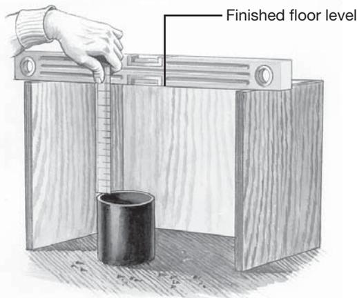
2. Measure the distance between the top of the connecting pipework and finished floor level.
