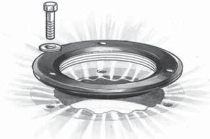
6. Where applicable, dress the membrane over the flange and into the sump of the body, ensuring that the membrane does not restrict the outlet; bolt the membrane clamping collar to the body – certain collars are reversible to increase height adjustability.
