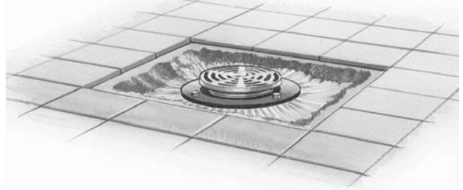
7. Fit grating, cover, or funnel with extensions, frame or collar as applicable; set top face flush and level with the finished floor using height adjustability features. Use a suitable, good quality sealant on all threaded joints to ensure a watertight assembly.
