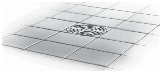
8. Infill or lay floor screed and apply final floor finish (e.g. tiles, marble, paviers, terrazzo) around the grating or cover.
