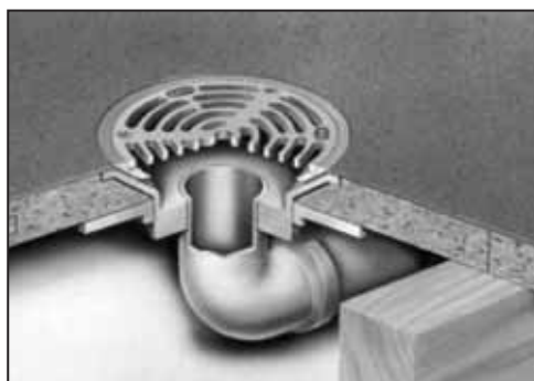
Watertight Drainage in a vinyl covered timber floor
